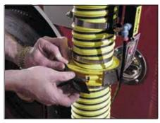
The safety disconnect coupling is to protect your investment from unexpected work place occurences, such as when a service technician forgets to remove the exhaust hose from the vehicle before moving it. The safety disconnect coupling will automatically separate to protect the vehicle and your exhaust system.
