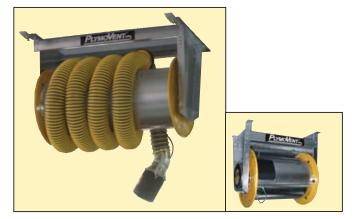
The model MHR is designed to retract the exhaust hose with an electric motor drive. When using the exhaust hose, press an up/down switch mounted on the wall or a key set mounted to the exhaust reel. The motor has an adjustable up/down limit switch to stop the hose at any desired level. When the exhaust hose is not in use, retract the hose to the ceiling.
