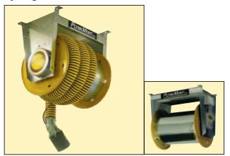
The model SER is designed to retract the exhaust hose with a spring operated retraction device. When you need to use the exhaust hose, pull down the hose and attach the nozzle to the vehicle. The hose will lock into place. When finished, remove the nozzle from the vehicle and pull down again, and the hose will smoothly be returned to the hose reel.
